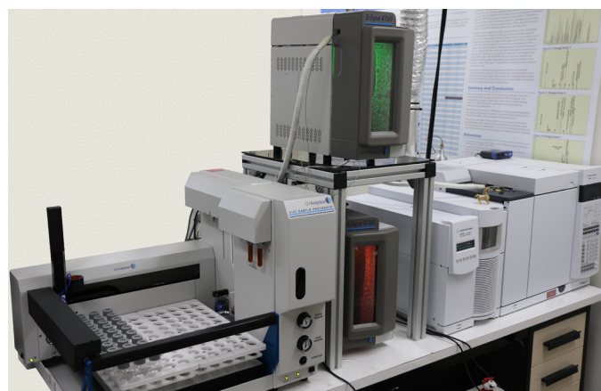
Figure 1. OI Analytical 4100 Autosampler and Eclipse 4760 Purge & Trap and Agilent 7890A/5975C GC/MS
